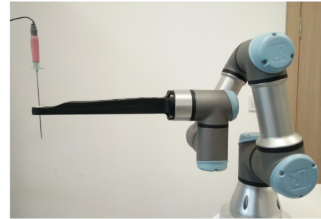
FIGURE 6 The extended end-effector of Universal Robots 3
